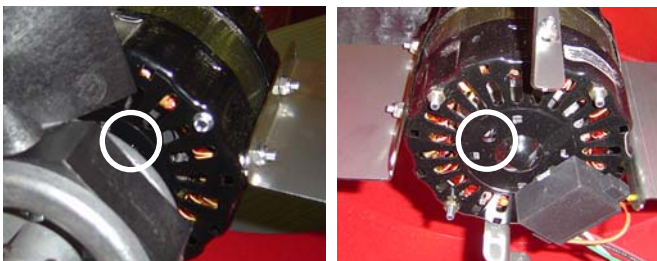
Figure 8: Oil hole locations. Access the oil holes by removing the protective grill(s) and turning the unit upside down.
