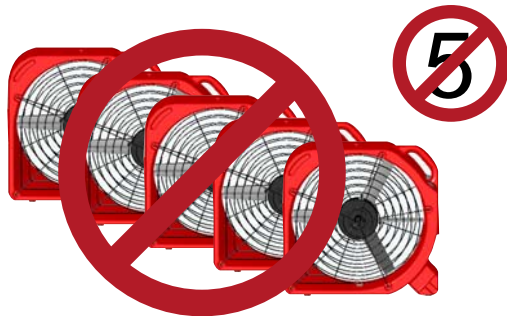
Figure 1: Too many AXIAL AIR MOVERS daisy-chained.
