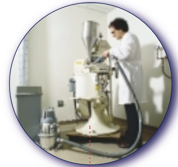
GM 80i removing excess powder from a tablet press during manufacture.
