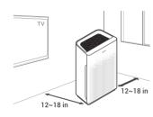
Allow 12 ~ 18 in. of space between TVs, radios, and other electronics Electromagnetic interference from certain electronics may cause product malfunction.
