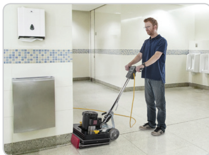
Baseboard cleaner, standard on the XP model, eliminates the need for getting down on your hands and knees or using a dedicated baseboard cleaning machine. (Optional on ST machine)
