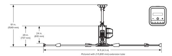
Wired Standard Control Height: 4.86 in. (123 mm) Width: 4.54 in. (115 mm) Depth: 1.3 in. (29 mm)
