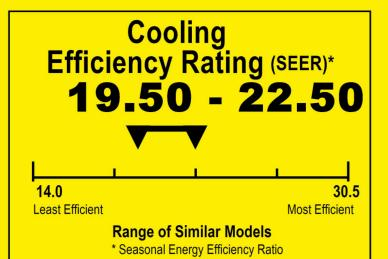
This system's effciency ratings depend on the coil your contractor installs with this unit. The heating efficiency rating varies slightly in different geographic regions. Ask your contractor for details.
