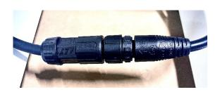
Connect the M16 ends together and tighten the screwing lock to secure the connection.
