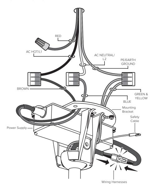
Fig. 11b: Wiring Diagram (With EMI Filter)
