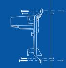
5 Using a Phillips-head screwdriver (G), screw the wall bracket into place. Turn clockwise on each of the four screws until vou feel a firm resistance.
