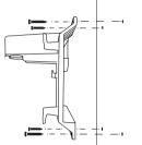
4 Using a Phillips-head screwdriver (G), screw the wall mount into place. Turn clockwise on each of the four screws until vou feel a firm resistance.
