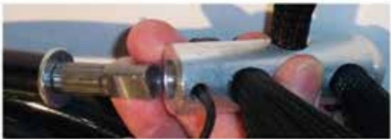
Attaching brush to cable
