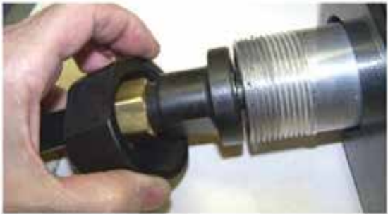
Attaching brush cable to connector
