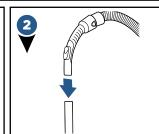
Connect the Hose Handle to the end of the Extention Wand and twist slightly to tighten.
