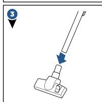
Connect the Multi-Surface Floor Tool to end of the extension wand and twist slightly to tighten.
