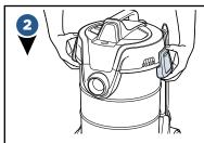
Undo the clips on both sides of the Top Cover and lift up to remove.
