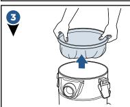
Remove the Large Fabric Filter by pulling up, holding both sides, and then setting it to the side.
