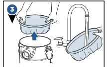
Remove the Large Fabric Filter and hand wash in cold water with mild detergent. Rinse well and air dry for 24 hours.
