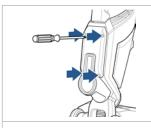
1. With a Phillips-head screwdriver, remove the 4 screws on the back of the machine. Lift off the back cover.
