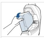
1. The Clean Water Tank is located on the back of the machine. To remove, use the finger groove at the top of the tank to grab and pivot the tank backwards.
