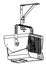
10. Loosen the screw to remove the wiring compartment/connection cover in the rear of the heater.
