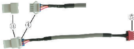
Fig. C: Schematic diagram of patch cord: Terminal ⑤ is the protection terminal ; connect terminal ③ to the terminal ① of connection wire ; connect terminal ④ to the terminal of wired controller of air conditioner
