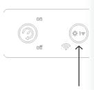
While the heater is plugged in and turned on, press and hold the wifi/sun symbol on control screen for 5 seconds. You should hear a beep and see a wifi symbol start blinking in a blue color
