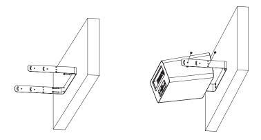
Different facing angles are available by choosing the holes to fix the handle onto the heater body.
