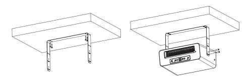
There are two positons from the ceiling are provided by choosing the installation hole of the handle
