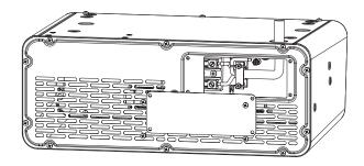
2. Put the cable with 10 gauge internal wires into the chamber through the hole on the top, the cable, connect L, N and Ground and hold by the cable by a clip inside the chamble.
