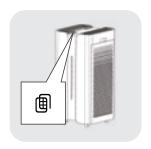
When the purifier indicator panel on the "reset filter" flashing lights, you need to replace the filter.
