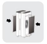
Put the new complex filter in the direction of the arrow to return to the product internally..
