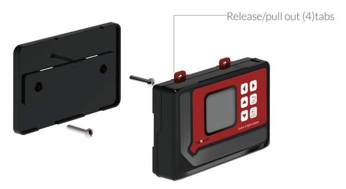
Determine where to locate the main controller. The controller comes with a simple to use DIN type bracket. Pull the 4 tabs outward to release the bracket from the unit, mount the bracket to a wall or surface, place the unit back on the bracket and press the 4 tabs back in to lock the unit in place.
