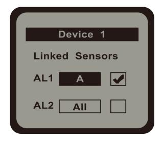
Use LEFT, RIGHT, UP and DOWN button to adjust the setting and press ENTER to confirm. The device station will be activated when the linked sensor/sensors detected a CO2 level over the related limit setting.
