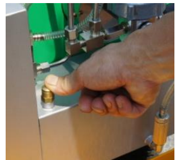
Directional Valve Turn right for Oil Based fogging
