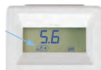
Successful pH 7 and pH 4 calibration
