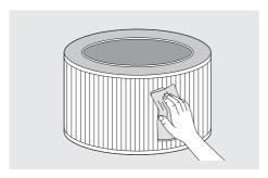
Gently brush off the collected dust on the surface of the prefilter with dry cloth, or vacuum cleaner for optimal performance.
