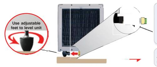
Screw female end of drain line onto Fral drain.
