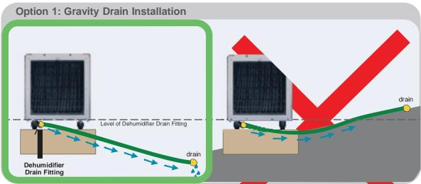
**IMPORTANT:** The drain hose must run downward and stay below the level of dehumidifier drain fitting.
