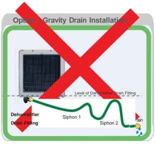
WARNING: Double siphon is not allowed because it not allow correct drainage of water
