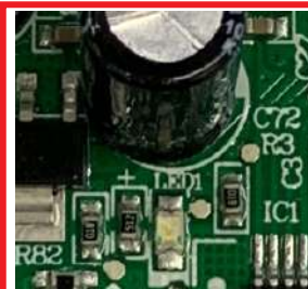
LED1: Drive failure indicator
