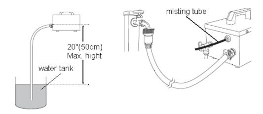
**TIPS!** A [Calcium Inhibitor Filter] can be connected between the tube and the faucet. It is a good habit to always has this filter included for quality water supply, and to prevent early clogging of the nozzle. The inhibitor filter is NOT included.
