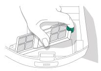
2 Make sure bin is upright, and over the trash, push the release tab to open the bin.
