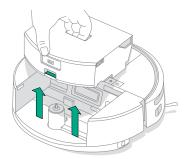
4 Remove the filter by pinching the tab and pulling the filter out.
