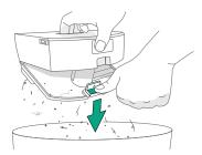
2 Remove water tank and mop pad, by pressing the tank release buttons on both sides of the robot to slide out.
