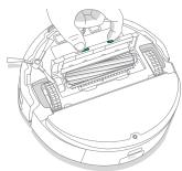
**4** Reinstall the multi-surface brush and brush cover in the robot.
