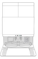
Solid White: When the robot is fully charged or in the process of charging. While the dock is automatically emptying the bin, during washing or drying cycles, and when the dock is in standby mode.
