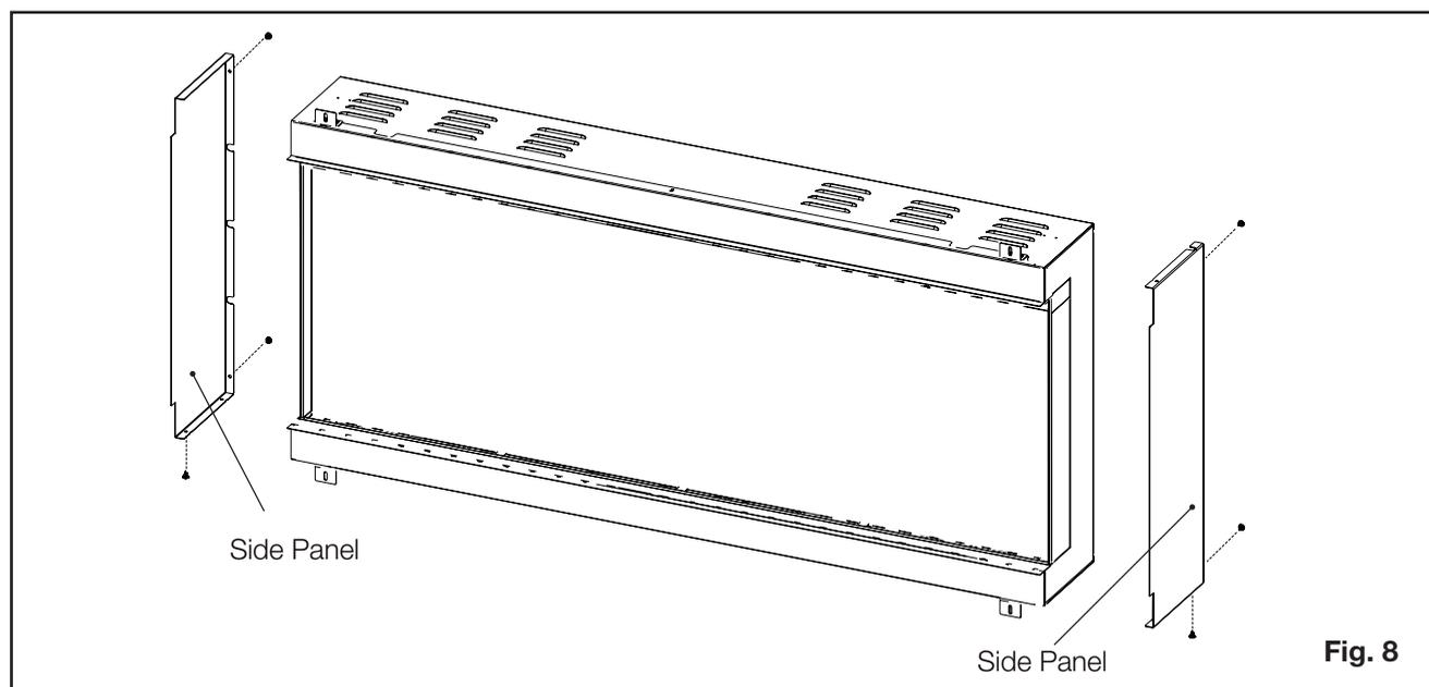
For an end wall enclosure with 2 sides (front and 1 side) install the top and bottom trims along with 1 C shaped panel and 1 flat panel to the respected side which are required to be open and closed.
