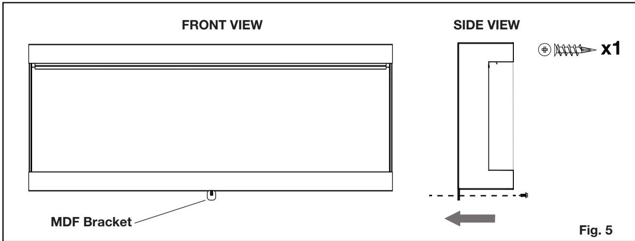
7. With the MDF bracket secured to the appliance, secure the MDF bracket to the wall using one screw (**Fig. 5**).
