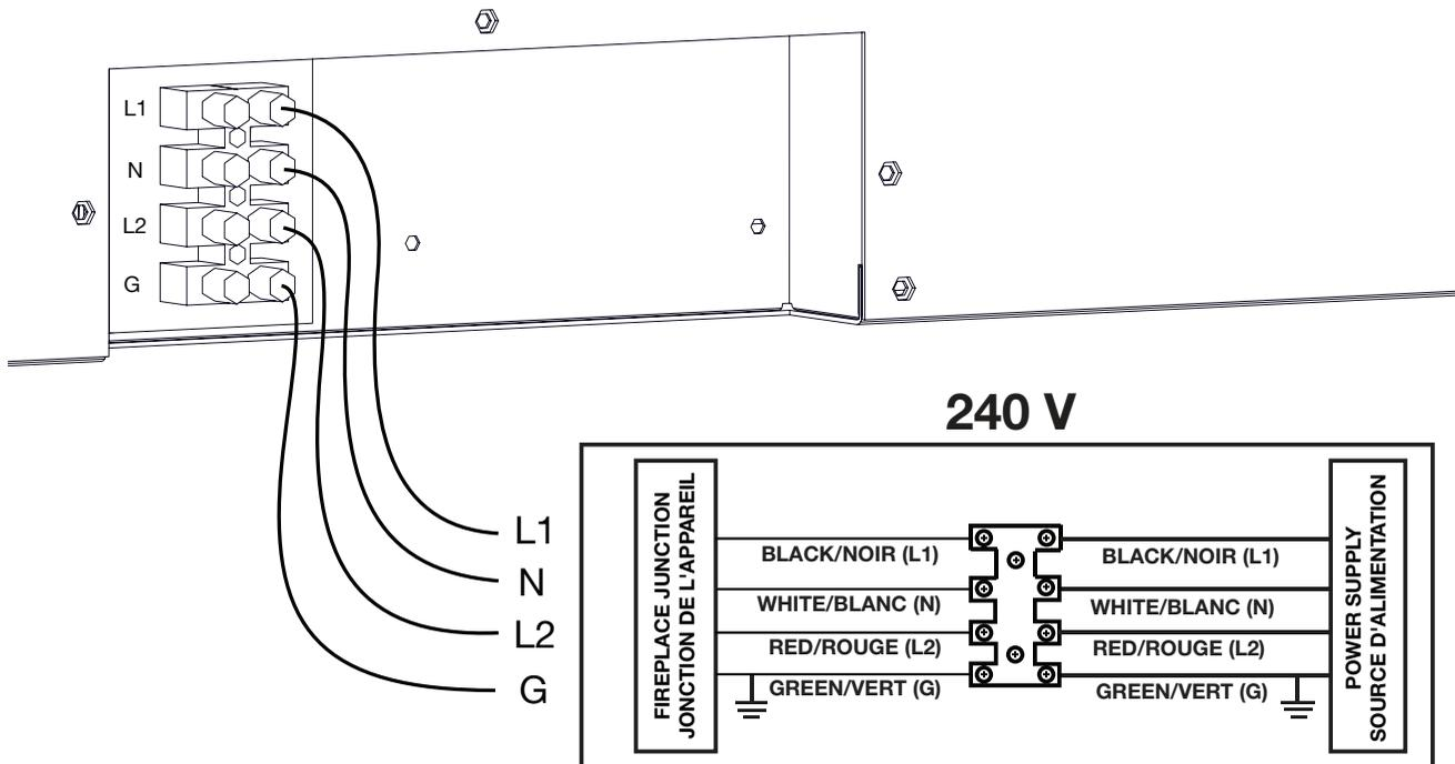
1. Insert Green or bare copper wire to the designated G Terminal. Tighten the screw.
