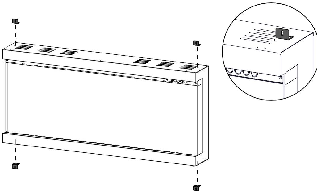
5. Insert the appliance into the rough framing by securing the screws (supplied) through the slotted holes on each securing bracket of the appliance into the rough framing. **(Fig. 7).**
