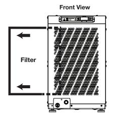
**Step 3** - Insert the new filter into the filter compartment and attach the magnetized filter door back into place, ensuring it covers the filter compartment completely. Be sure the arrows on the filter are facing into the dehumidifier.
