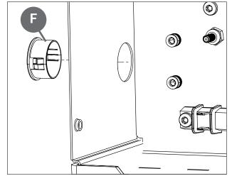
**Step 5**. Route wires through 7/8" hole and secure using the clamps intended for conduit or cable. There is a hardwire jumper kit included with the unit.
