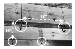
**Step 3:** Two ropes are installed into the four rachets. Lift tab on rachet to release if the rope is pulled to far. Hook snap hook on the ratchet pulley to the first installed D-ring and pass the other end of the rope with the ratchet pulley under the dehumidifier lining up the rope in the channel in the base of the dehumidifier. Hook the snap hook into the second D-ring installed on the joist. Complete these same steps on the other side of the dehumidifier.
