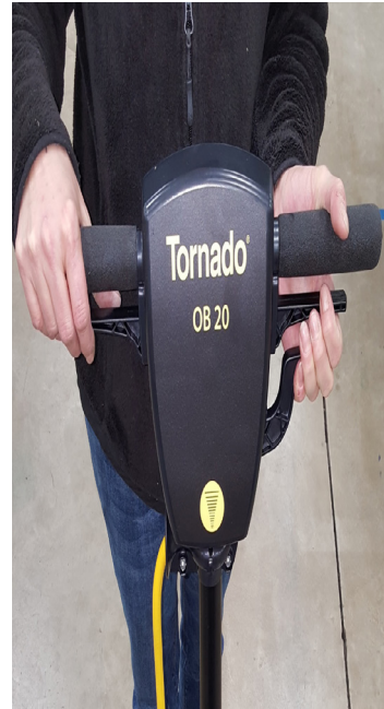
Adjusting handle height using the handle adjustment lever
