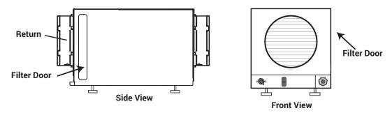
Step 2: Remove the filter by gently pulling straight out of the unit. Insert new filter by gently pushing it straight into the unit. Make sure the AIR FLOW arrow on the filter is pointing into the unit.
