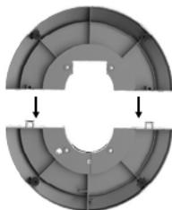
2. Feed the power cord through the center hole on the base.
