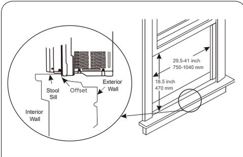
3. All supporting parts must be secured to firm wood, masonry, or metal.
