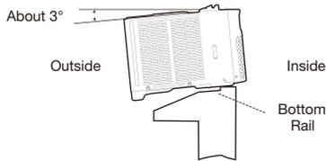
**NOTE:** The air conditioner should be tilted about 3° to allow for better drainage of condensation and rainwater. Using a level, measure about 1/3 bubble for the correct slant.
