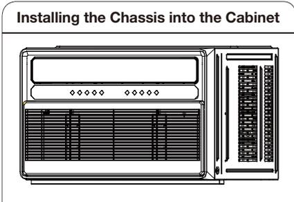
Push the chassis into the cabinet. Reinstall the screws of cabinet, and reattach the front facelate, front panel, and air filter.
