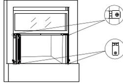
**NOTE:** Fix the upper screws first, then the lower screws. When open the window, be sure that all the screws are fastened tightly.
