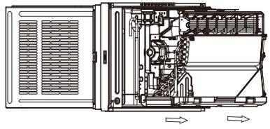
Hold the cabinet while pulling on the base handle to install the unit.
