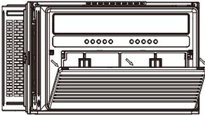
Pull down the front panel and remove the filter. Lift the front front panel upwards and remove from the air conditioner.
