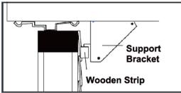
5. Screw the cabinet to the wooden frame using shims as below with 7 long Hex-head screws, remember to maintain proper slope for water elimination.
