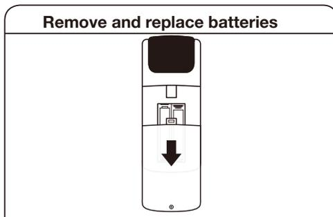
Use a small Phillips screwdriver to loosen the battery cover screw. Slide the battery cover down with two thumbs to remove. Remove and properly dispose of old batteries, then replace with two new AAA batteries. Replace the battery cover and tighten the screw.
