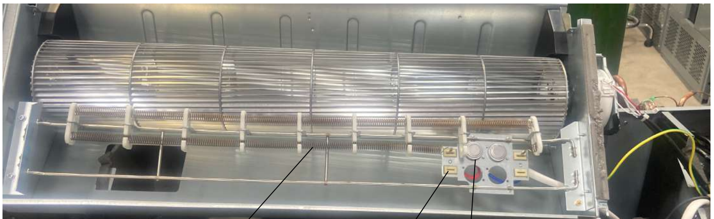
Heater Coil Heater Wire Terminals Limit switches
