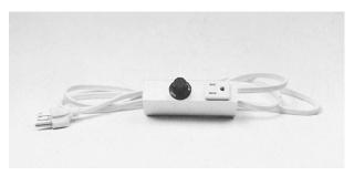
An optional portable thermostat is available for use with any WorkWarmer™ "plug in" heater 120 Volt, 10 amps, 1200 watt maximum capacity. Snap action switching. "Hi - Lo" control. White plastic case and 5' white cord. Velcro tape is attached to the thermostat for mounting.
