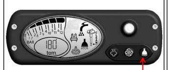
Increase / Decrease water injection by pushing and holding the button on the console.
