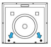
5. Place the two included adhesive discs on the two small circles on the back of the unit.
