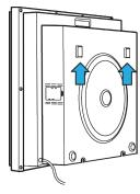
6. Once the bracket has been properly affixed to the wall, slide the unit down onto the bracket's hooks slowly. Align the unit's bracket pockets with the hooks to assure a secure installation.
