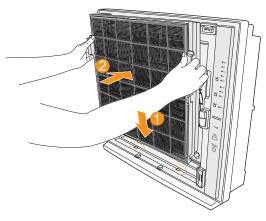
10. Reattach the front panel by latching the top hooks, then securing the bottom of the panel.
