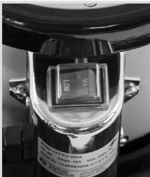
Dual speed 185/330 rpm DC motor.
