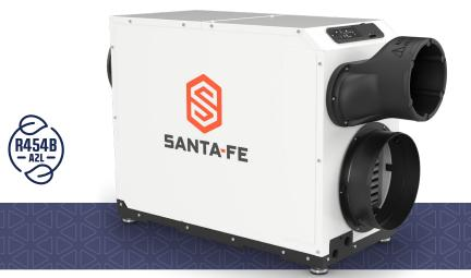
The **Ultra V100** is a high-performance ventilating dehumidifier with vertical or horizontal airflow discharge. The unit provides high-efficiency water removal and features an 8" ventilation duct to increase outdoor air intake to help meet ASHRAE 62.2 requirements.
