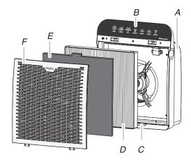
A. Mainframe assembly D. HEPA filter
